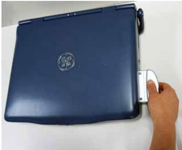
Figure 3-34. Probe connection to LOGIQ V2/LOGIQ V1
