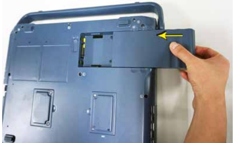
Figure 3-13. Place the battery on the bottom cover
