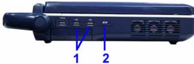
Figure 15-13. USB ports on the left side
