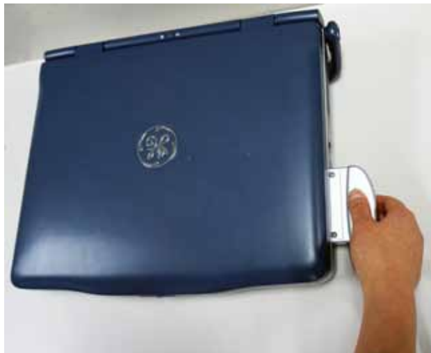
Figure 3-37. Probe disconnection from LOGIQ V2/LOGIQ V1
