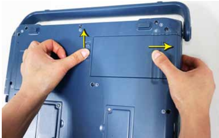
Figure 3-15. Unlock and push the battery
