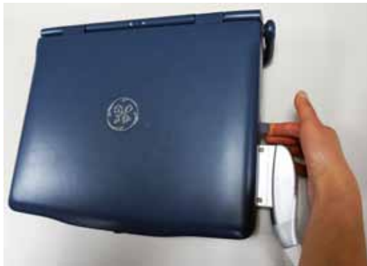
Figure 3-35. Probe connector locking lever
