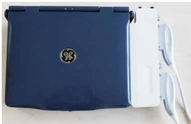
Figure 3-42. 2-Probe Port Adapter connection 5
