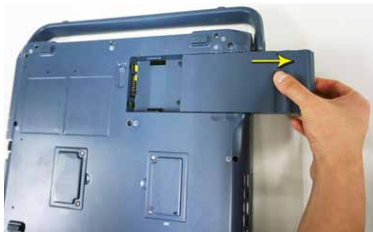
Figure 3-16. Remove the battery
