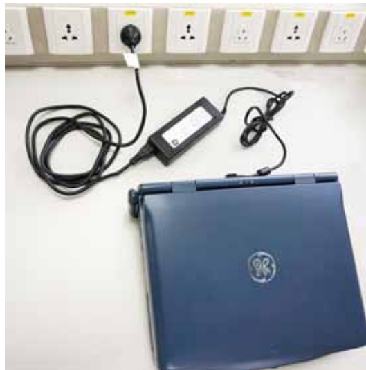
Figure 3-22. Connect the system to the electrical supply
