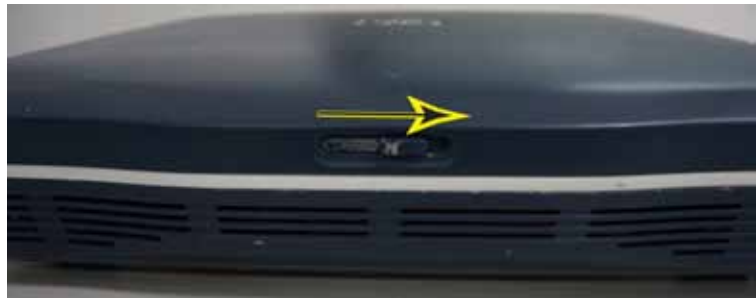
Figure 3-31. Unlock the LCD Monitor
