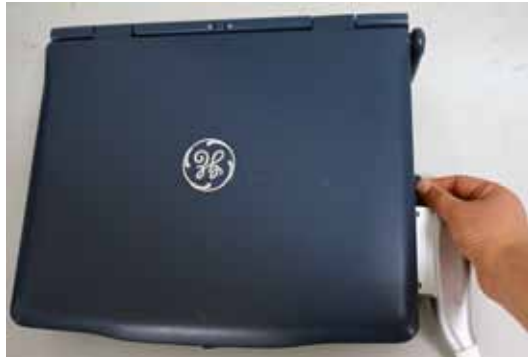
Figure 3-36. Probe connector unlocking lever
