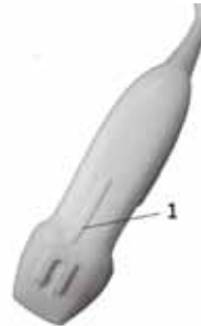
Figure 17-1. Orientation Marking on Probe (Example)
