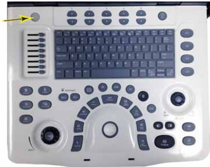
Figure 3-24. Power On/Off Switch Location
